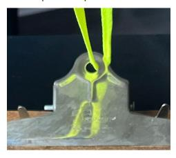
B. Pass the end of the rope through the loop.
