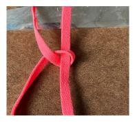
D. Tighten the rope to complete a two half-hitch knot also known as a double half hitch knot.
